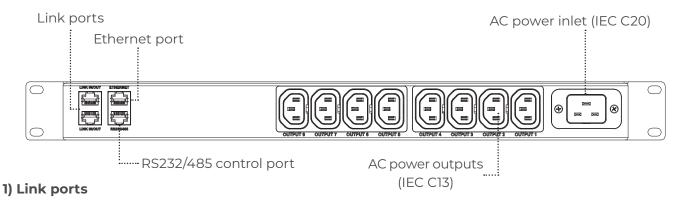
Up to 20 PSQ108 intelligent power sequencer devices can be daisy chained using link ports. Each RJ45 socket can be either an input or an output.
