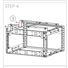
When hooked, secure the rack into the bracket by inserting and tightening two bolts into the provided mounting holes as indicated in above image. This prevents the rack from falling down by accidential touching, vibration or other impacts.
