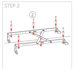
Mount the bracket to the desired mounting location on the ceiling. Use the included anchor bolts or other fasteners depending on the mounting location or surface. Always make sure the surface can structurally support the weight of the bracket including the rack weight.
