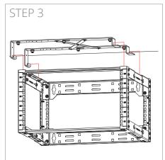
Pre-assemble the equipment in the rack, and hook the rack into the bracket as indicated in above image.
