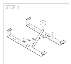
Assemble both beams with the correct distance in between, using the 'X' support. The distance is depending on the required depth of the rack
